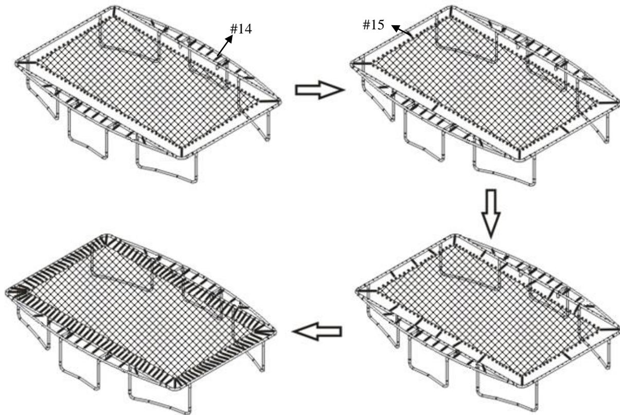
D. If you notice that you have skipped a hole and V Ring connection, recount and remove or attach any springs required to maintain the count of springs.
